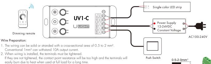
Note: The output power of a constant voltage power supply should be at least 1.2 times that of the output load (light strip), otherwise the full power output of the load can easily cause automatic flickering or shaking of the light.
