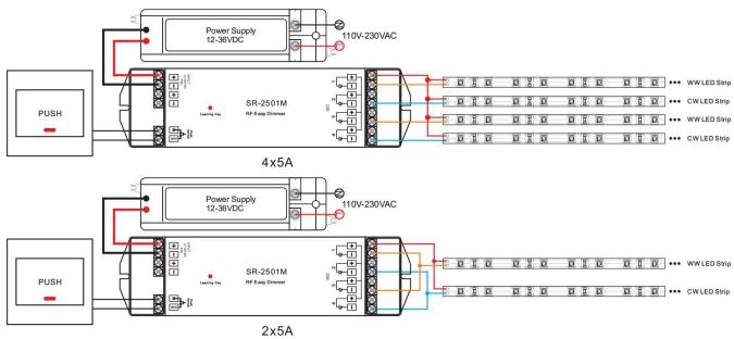
Receiver Connection Diagram for Multiple Units
