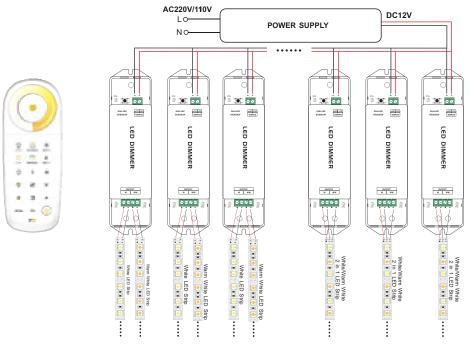
2. Each Receiver is Powered by One Power Supply Independently:
