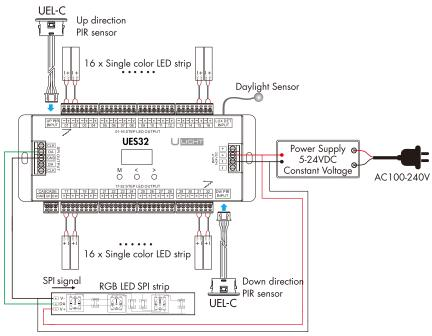
Connect the UES32 sensor stair light controller to two laser sensor head, which are installed at the top and bottom of the stairs. Set the delay time of the laser sensor head to 2s (default).
