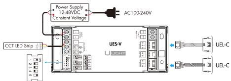
The UES-V constant voltage controller is connected to two laser sensor head which are installed on each side of the corridor.
