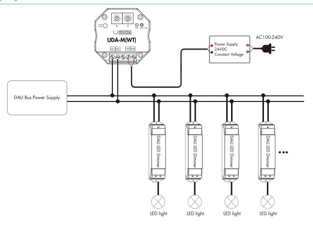
Note: When UDA-M(WT) is working, because the power consumption of the WiFi module is too large, it cannot be powered by the DALI bus power supply.
