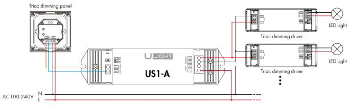
• Triac dimmer (with null and live line) + Multiple triac power amplifiers + Multiple triac dimming drivers
