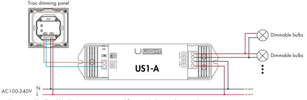
• Triac dimmer (with null and live line) + Triac power amplifier + Multiple triac dimming drivers
