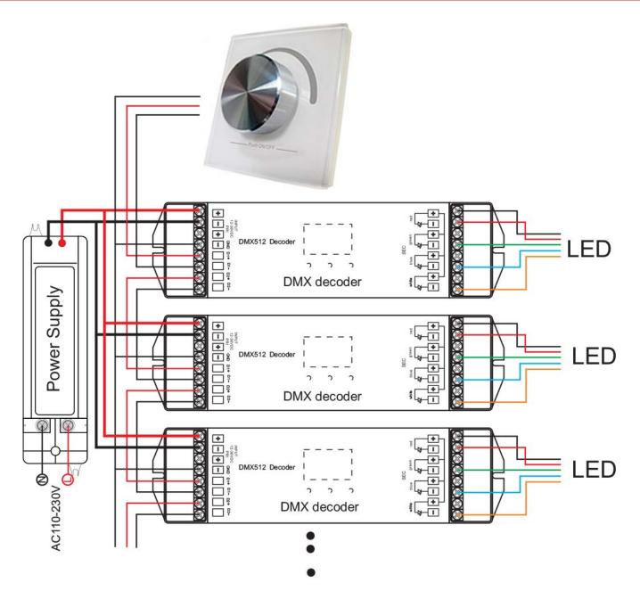
**Set Zones by DMX Addresses on decoders,** please set the connected DMX512 decoders' addresses as below:
