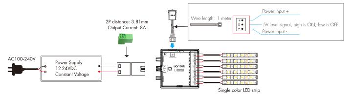
• Power supply using cabinet constant voltage power supply + junction box
