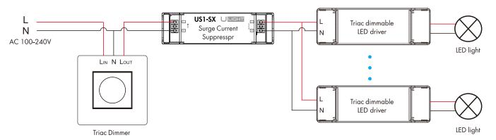
Note: It is recommended that the total power of the connected LED dimmable drivers or LED dimmable luminaires load does not exceed 2000W and the total working current does not exceed 8A.
