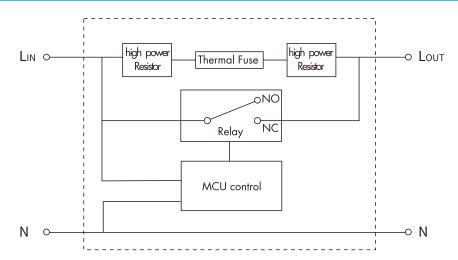
The moment the product is powered up, two  $7.5\Omega$  high power resistors are connected in series between LIN and LOUT to reduce the load power-on surge current. After about 40ms, the relay switch will be engaged and the LIN and LOUT will go through.
