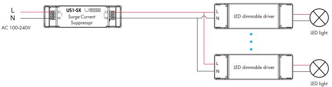
2. Surge current suppressors for use in series with triac dimmers to connect one or more triac dimmable LED drivers
