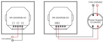
2)Receiver Connection Diagram for Multiple Units
