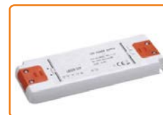
LED power supply SLIM 30W • Pri: 180-264V~50/60Hz • Sec: 12V DC eff, 2,5A • max load 30W • short circuit protection • size: 159x59x18mm
