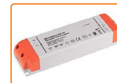
LED power supply 60W • Pri: 220-240V~50/60Hz • Sec: 12V DC eff, 5A • max load 60W • short circuit protection • size: 180x52x30mm
