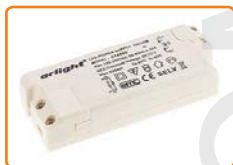
LED power supply 10W • Pri: 170-264V~50/60Hz • Sec: 12V DC eff, 830mA • max load 10W • short circuit protection • size: 102x39x20mm
