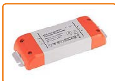
LED power supply 15W • Pri: 220-240V~50/60Hz • Sec: 12V DC eff, 1,25A • max load 15W • short circuit protection • size: 123x45x19mm
